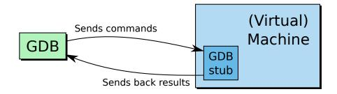
Because it has been generally used to debug kernels on physical machines using the serial link, the protocol involved in the comunication with the GDB stub is called the Remote Serial
