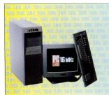
The Leo 386/16, from Computer Systems Corp., is an atfordably priced, zerowait-state tower system. The use of mostly standard components in a sturdy case is commendable, but the front-panel turbo and reset buttons look alike and are dangerously close to each other.
